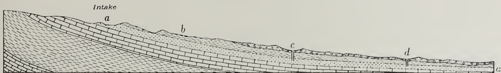
FIG. 25.—Diagram showing conditions necessary for an artesian basin; a is a porous layer, b is an impervious layer that traps water in a , and c and d are flowing wells.
